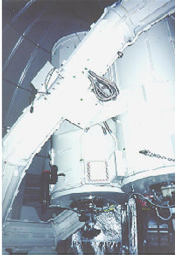
**MWO binocular telescope showing V-tube (left) and IR-tube (right)**
